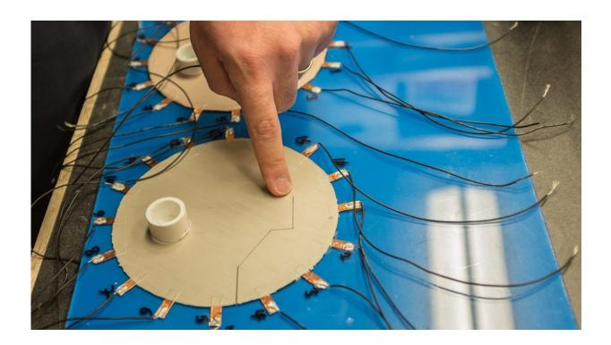
The multi-functional, multi-layer sensing skin is applied to a polymeric substrate with a physical crack and a reservoir for exposing the sensing skin to aggressive ions. Credit: Julie Williams Dixon.
