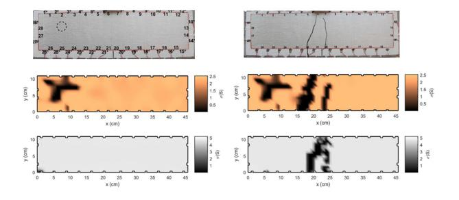
An example of testing a multi-layer sensing skin for detecting chlorides and cracking. The top row shows photographs of the sensing skin on a concrete beam surface before and after cracking the beam. In the top left photograph, the dashed circle indicates an approximate location of an embedded chloride solution reservoir. The second and third row illustrate the EIT reconstructions of
