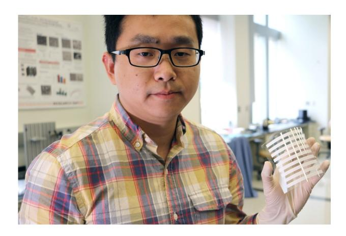
Post-doctoral researcher Congcong Wu, who is working in the lab of Shashank Priya, the Robert E. Hord Jr. Professor of Mechanical Engineering, holds up a layer of the flexible solar panel the group is working on. The process to adhere a thin film of titanium oxide to the panel takes less than 10 seconds using screen-printing technology. Credit: Virginia Tech
