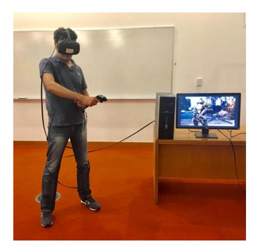
The "MoVR" system allows for cable-free virtual-reality gaming, eliminating the possibility of users tripping over cords. Credit: MIT CSAIL
