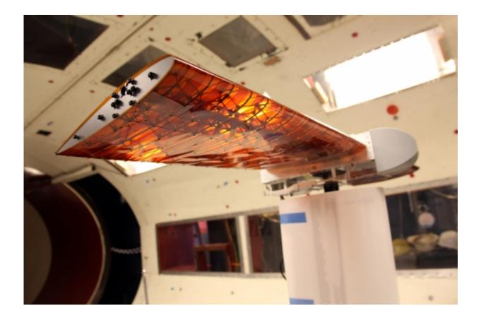
In the team's new approach, the whole shape of the wing can be changed, and twisted uniformly along its length, by activating two small motors that apply a twisting pressure to each wingtip. Credit: Kenneth Cheung/NASA
