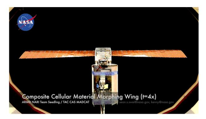
A test version of the deformable wing designed by the MIT and NASA researchers is shown undergoing its twisting motions, which could replace the need for separate, hinged panels for controlling a plane's motion. Credit: Kenneth Cheung/NASA
