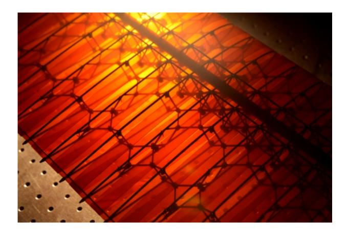
The basic principle behind the new concept is the use of an array of tiny, lightweight structural pieces, which Neil Gershenfeld, director of MIT's Center for Bits and Atoms (CBA), calls "digital materials," that can be assembled into a virtually infinite variety of shapes. Credit: Kenneth Cheung/NASA
