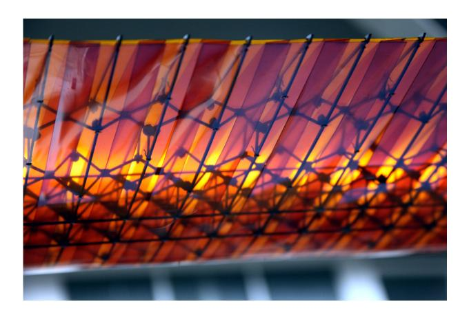
A newly developed wing architecture could greatly simplify the manufacturing process and reduce fuel consumption by improving the wing's aerodynamics. It is based on a system of tiny, lightweight subunits that could be assembled by a team of small specialized robots, and could ultimately be used to build the entire airframe. Credit: Kenneth Cheung/NASA
