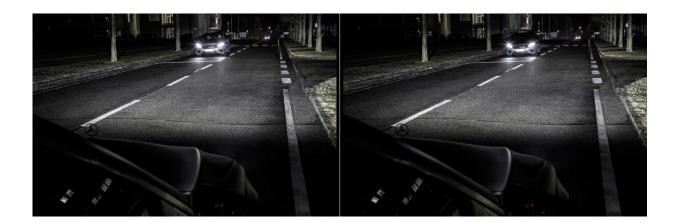
The new HD projector technology from Mercedes-Benz uses sensors on the vehicle to identify other road users and ideally adapt the light distribution to the environment. In this process, drivers and front passengers of oncoming vehicles
