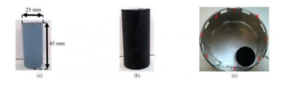
(a) A plastic rod was used as a prosthesis surrogate. (b) The rod was coated with a pH-sensitive thin film sensor and (c) tested experimentally using a prototype ECT mapping system. Credit: University of California - San Diego
