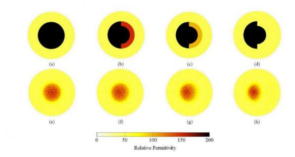
During simulations, a prosthesis was assumed to be embedded in human tissue (a). Figures b to c show how infection changes the electrical properties in a semicircular region at the tissue-prosthesis interface. (e) to (h): electrical maps from ECT simulations showed that the technique was able to capture changes due to degradation (or infection). Credit: University of California - San Diego
