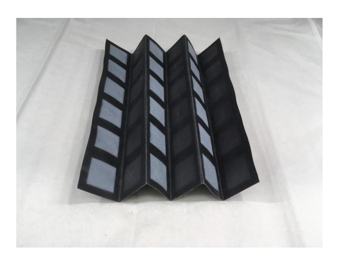
Researchers at Binghamton University, State University of New York have created a bacteria-powered battery on a single sheet of paper that can power disposable electronics. Credit: Seokheun
