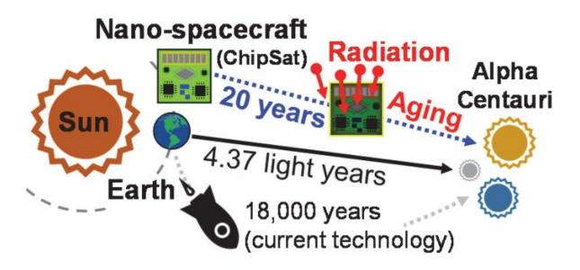
A nano-spacecraft such as ChipSat, which consists of solar cells and functional blocks in a printed circuit board, would face a high risk of damage from radiation and aging issues on a flight into deep space. Especially, most of functional blocks such as microcontroller, memories, sensors, and communication system are semiconductor-based chips. Credit: D.-I. Moon et al.
