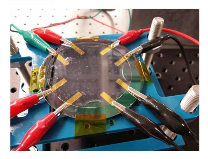
The pectin film was integrated into a synthetic-skin-like material. This square patch of artificial skin was able to sense temperature variations across the pixelated matrix. Credit: Di Giacomo et al., *Sci. Robot.* 2, eaai9251 (2017)
