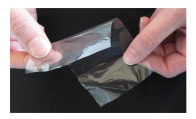
This thin pectin film is a strong temperature sensor. Credit: Di Giacomo et al., *Sci. Robot.* 2, eaai9251 (2017)
