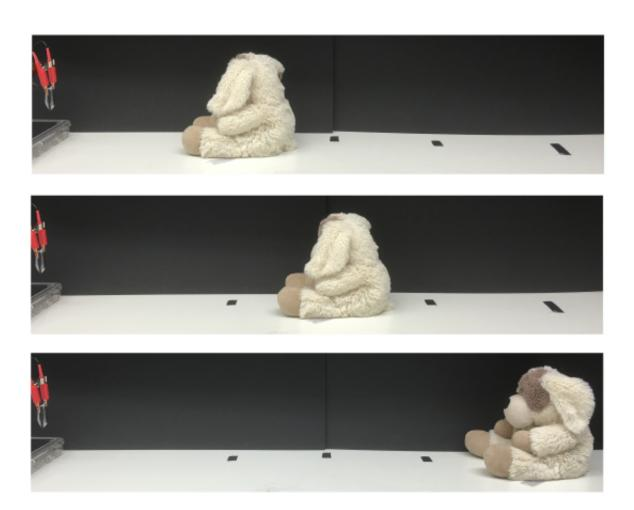
A teddy bear warmed up to 37 degrees Celsius (98.6 degrees Fahrenheit) was placed some distances away from the pectin film, which could sense it at up to one meter away. Credit: Di Giacomo et al., *Sci. Robot.* 2, eaai9251 (2017)
