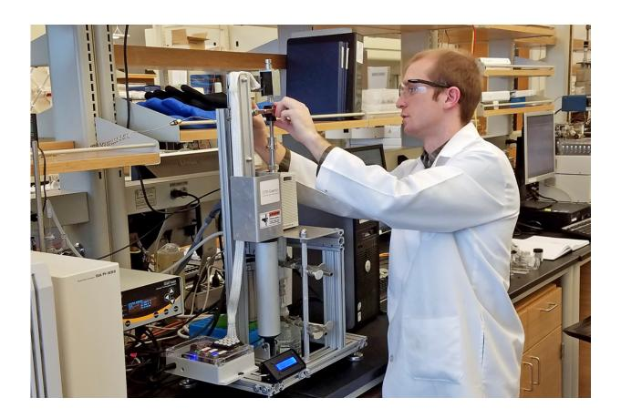
Jake Lindstrom, an Iowa State graduate student in mechanical engineering, loads a biomass sample into a Controlled Pyrolysis Duration (CPD)-Quench reactor. The system helps scientists better understand the products and mechanisms of fast pyrolysis. Credit: Robert Mills/Iowa State University Bioeconomy Institute.
