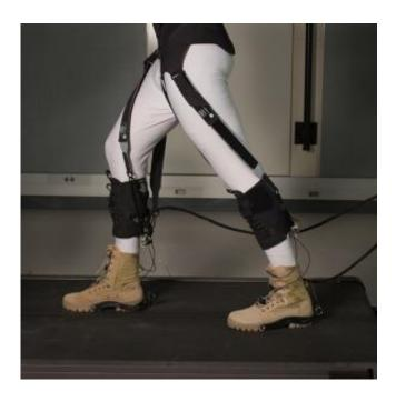
The exosuit's soft textiles strategically position the actuating cables that assist with the ankle motion at the back of the lower legs, and, through additional straps, transfers energy produced at the ankle to the front of the hip to also assist with the gait's hip motion. Credit: Wyss Institute at Harvard University
