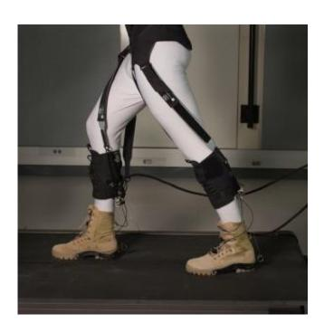
The exosuit's soft textiles strategically position the actuating cables that assist with the ankle motion at the back of the lower legs, and, through additional straps, transfers energy produced at the ankle to the front of the hip to also assist with the gait's hip motion. Credit: Wyss Institute at Harvard University
