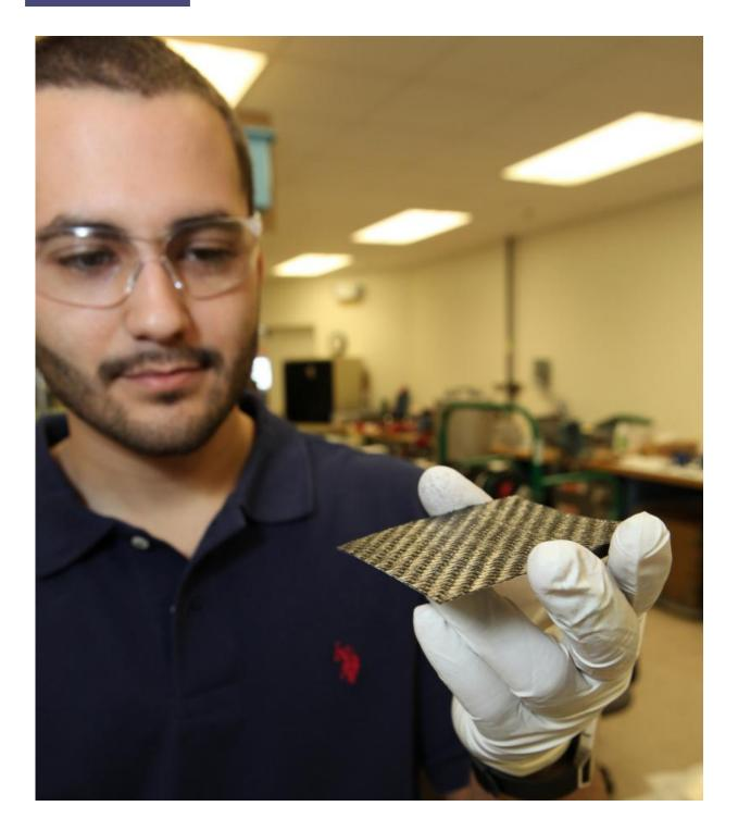
Daniel Perez, Ph.D., a graduate student from the University of Miami, displays a piece of the prototype structure for a new solid-state battery in the Prototype Laboratory at Kennedy Space Center in Florida. The size of the battery is so small that it could be a prime candidate for use in microsatellites, including CubeSats. Researchers at Kennedy are collaborating with experts at the
