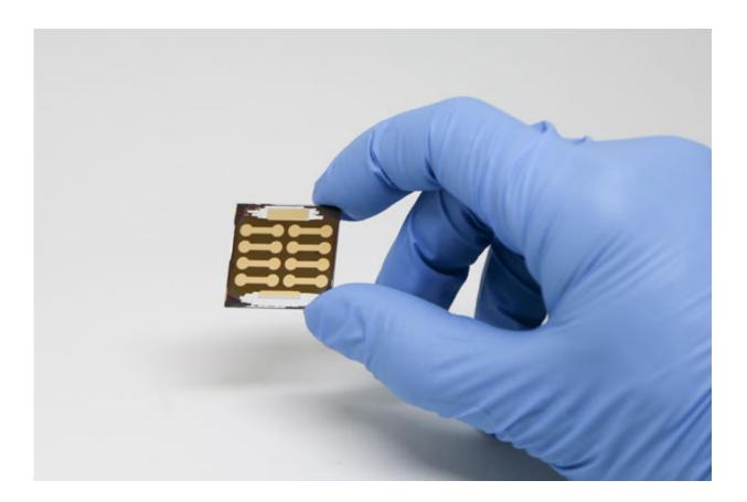
The new perovskite solar cells have achieved an efficiency of 20.1 per cent and can be manufactured at low temperatures, which reduces the cost and expands the number of possible applications. Credit: Kevin Soobrian
