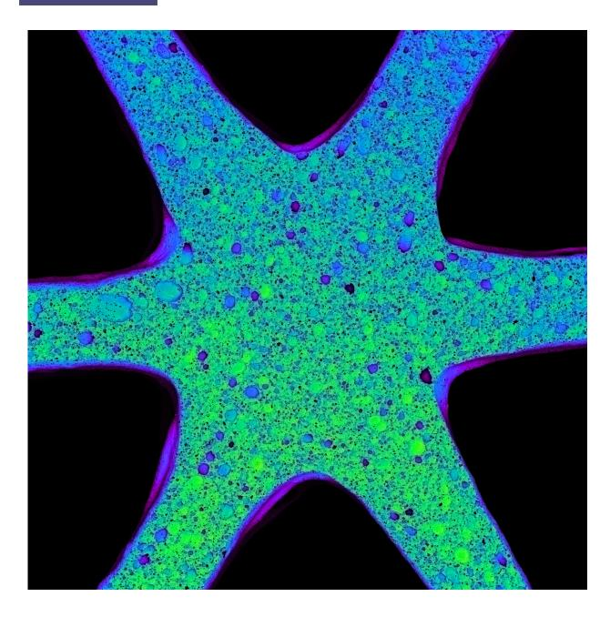
Close up image of one node of the triangular honeycomb. The structure, which consists of air surrounded by ceramic, can be designed with specific porosity. Credit: James Weaver/Wyss Institute
