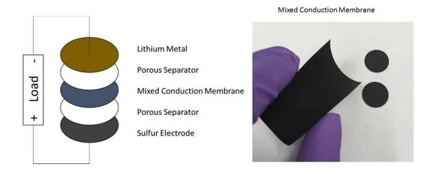
Lithium-sulfur battery with Mixed Conduction Membrane barrier to stop polysulfide shuttling. Credit: Sri Narayan and Derek Moy
