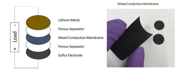
Lithium-sulfur battery with Mixed Conduction Membrane barrier to stop polysulfide shuttling. Credit: Sri Narayan and Derek Moy
