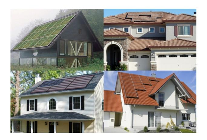
Founded at the MIT Sloan School of Management, Sistine Solar creates custom solar panels designed to mimic home facades and other environments, as well as display custom designs, with aims of enticing more homeowners to install photovoltaic systems. Credit: Sistine Solar
