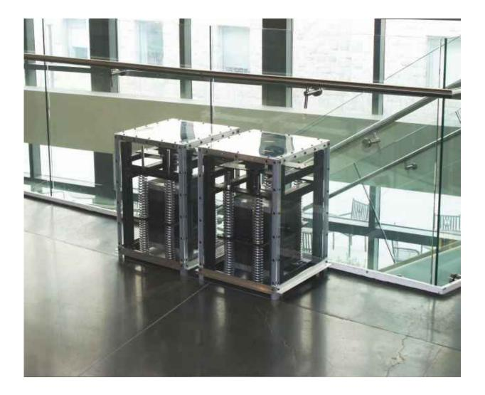
Easy to set up, tune, and move, the PTMD can be placed in areas with excessive vibrations, hidden away in a cupboard, or integrated into a building's design. Credit: Virginia Tech
