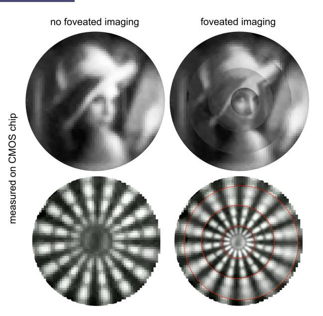
Experimental comparison of foveated and non-foveated imaging. The top images are of a commonly used test image called "Lena"; the foveated image shows increased detailed around the woman's eye. The bottom images demonstrate foveated imaging performance using a Siemens star test target. Credit: Simon Thiele, Kathrin Arzenbacher
