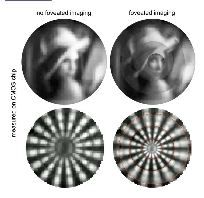
Experimental comparison of foveated and non-foveated imaging. The top images are of a commonly used test image called "Lena"; the foveated image shows increased detailed around the woman's eye. The bottom images demonstrate foveated imaging performance using a Siemens star test target. Credit: Simon Thiele, Kathrin Arzenbacher
