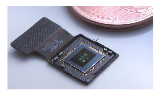
Image sensor and lens size comparison. Credit: Simon Thiele
