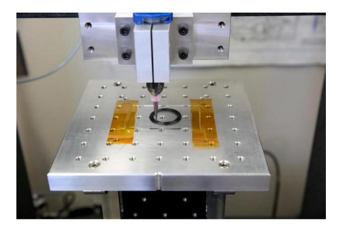
A carbon fiber composite ink extrudes from a customized direct ink writing (DIW) 3D printer, eventually building part of a rocket nozzle. Credit: Lawrence Livermore National Laboratory
