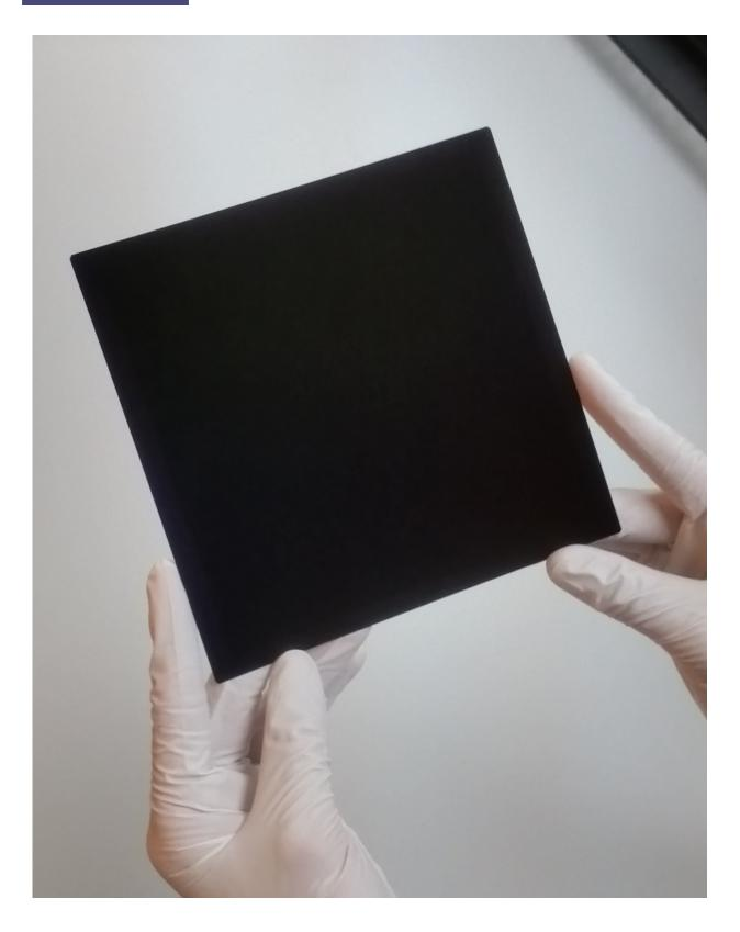
The photograph of HJ-IBC cell developed in Photovoltaic & Thin Film Research
