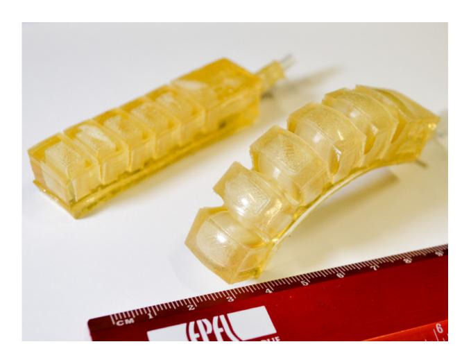
Edible soft pneumatic actuator developed in this study. (left) actuator in the nonpressurized state. (right) actuator in a pressurized state. Credit: arXiv:1703.01423 [cs.RO]
