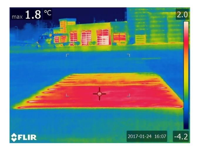
A thermal image of the heated airport pavements. Credit: Iowa State University
