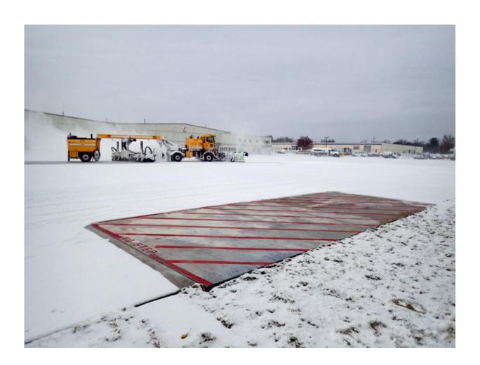
Iowa State engineers don't need a plow to clear snow from the heated test slabs they installed at the Des Moines International Airport. Credit: Halil Ceylan
