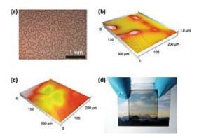
(a) Optical microscopy image of the commercial substrate that consists of a random mesh-like silver network on PET. Optical confocal microscopy images of the laminate electrode when coating with a ~450 nm thick (b) and ~1.3 um thick (c) PEDOT:PSS:sorbitol film. For small film thicknesses (b), the metal network is not fully covered. (d) Photograph of the semitransparent, laminated cell. Credit: Mohammed Makha et al
