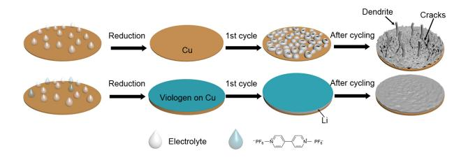
Illustrations of the design principles of using methyl viologen to form a stable coating to allow the stable cycling of lithium metal. Credit: UC Riverside
