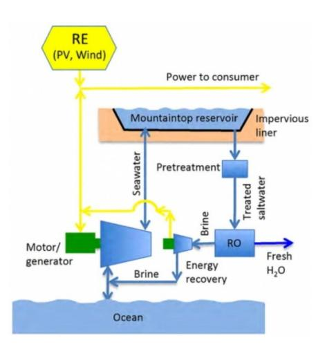
An integrated pumped hydro reverse osmosis (IPHRO) system produces both freshwater and electric power from renewable energy sources, such as solar power and wind power, by combining a pumped hydro energy storage system with a reverse osmosis desalination plant. Credit: Alexander Slocum
