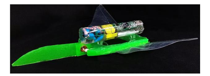
Something's fishy about this manta-ray-like robot. Perhaps it's the fact that it uses water as a conductor for dangerously high-voltage electrical energy? This system safely bent the robot's flexible layer and helped it flap its fins. Credit: Li et al. 2017;3:e1602045
