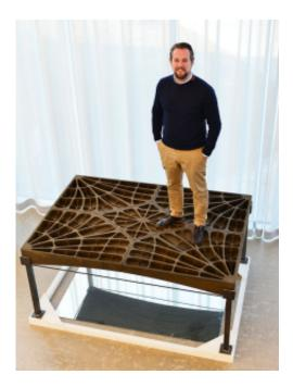
Holding firm – even without steel reinforcement: Philippe Block stands on a floor prototype printed using sand. Credit: ETH Zürich / Peter Rüegg
