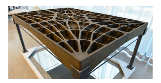
The construction of the unreinforced flooring, which is made up of individual slabs, takes its inspiration from Gothic cathedrals. Credit: Peter Rüegg / ETH Zurich
