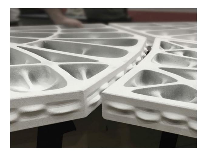
The individual slabs are joined together without mortar. Credit: Block Research Group
