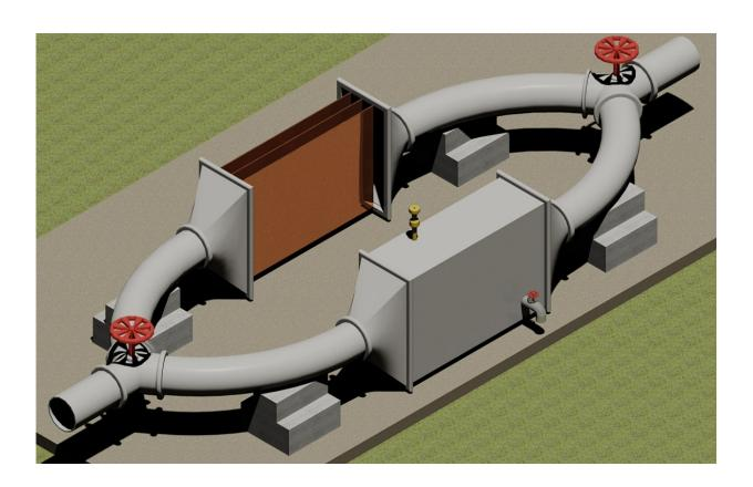
Artist's rendering of a prototype device that would electrokinetically remove asphaltenes from crude oil near the point of production Credit: Yao et al., 2015, Department of Petroleum Engineering, University of Houston
