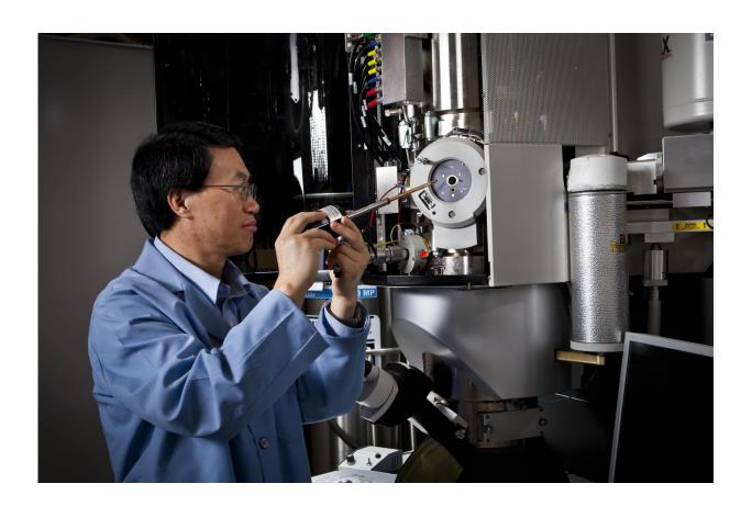
PNNL researcher Chongmin Wang and colleagues have developed the first step-by-step explanation of how a lithium-air battery forms bubbles, which expand the battery and create wear and tear that can cause it to fail. The research was aided by an environmental transmission electron microscope (shown here), which enabled the creation of a first-of-a-kind video that shows bubbles inflating and later deflating inside a nanobattery. Credit: Pacific Northwest National Laboratory
