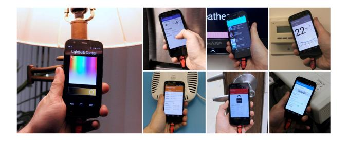
Example full-screen applications. Clockwise from left: lightbulb, refrigerator, television, thermostat, projector, door lock, and wireless router. Credit: Robert Xiao, et al.
