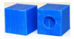
In the CAD model on the left, the deliberately embedded sphere disappears showing that the part is printed as high quality solid block when the right conditions are used. In the block on the right, the embedded sphere prints as a void if the required printing conditions are not used, giving that part lower strength. Credit: NYU Tandon School of Engineering
