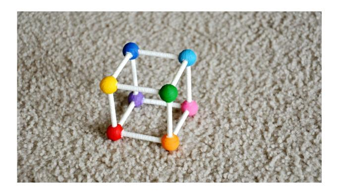
Researchers at North Carolina State University have developed a user-friendly, inexpensive controller for manipulating virtual objects in a computer program in three dimensions. Called CAPTIVE, the device allows users to manipulate objects more quickly -- with less lag time -- than existing technologies. Credit: Zeyuan Chen
