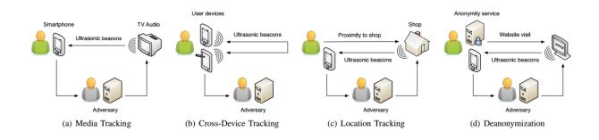
Examples of different privacy threats introduced by ultrasonic side channels. (a) Ultrasonic beacons are embedded in TV audio to track the viewing habits of a user; (b) ultrasonic beacons are used to track a user across multiple devices; (c) the user's location is precisely tracked inside a store using ultrasonic signals; (d) visitors of a website are de-anonymized through ultrasonic beacons sent by the website. Credit: Daniel Arp, et al.
