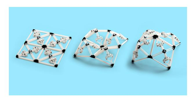
This object is printed flat (left) and can later be altered in two stable and loadbearing forms (middle and right). Credit: ETH Zurich / Tian Chen
