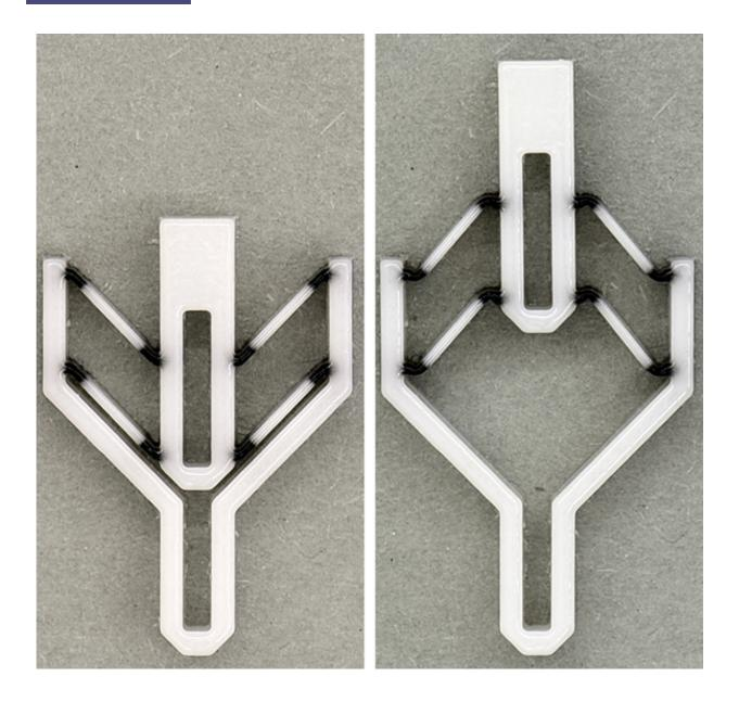
A single actuating element in its stable (left) and load-bearing (right) state. It consists of a rigid (light) and elastic (dark) polymer. Credit: Chen et al. Scientific Reports 2017
