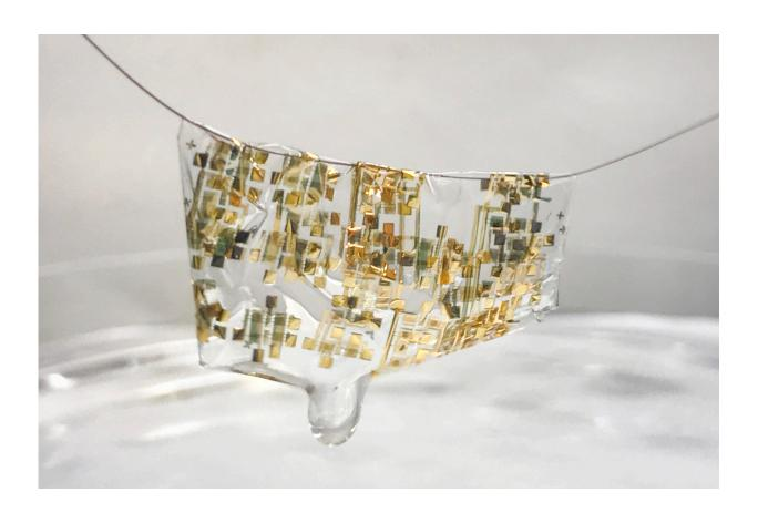
A newly developed flexible, biodegradable semiconductor developed by Stanford engineers shown on a human hair. Credit: Bao lab
