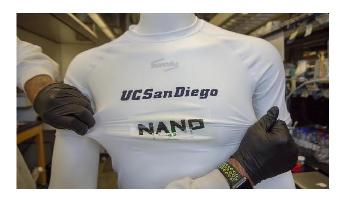
The stretchable batteries were printed on fabric for this demonstration. They make up the word NANO on the shirt and are powering a green LED that is lit in this picture. Credit: Jacobs School of Engineering/UC San Diego
