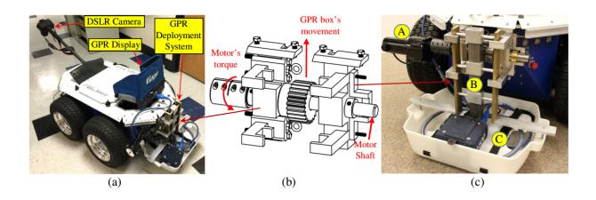
Autonomous robotic system for bridge deck inspection: (a) System overview; (b) Schematic of GPR deployment system; (c) Details of GPR deployment system: A - Motor, B - Gear shaft, C - GPR box. Credit: arXiv:1704.04663 [cs.RO]
