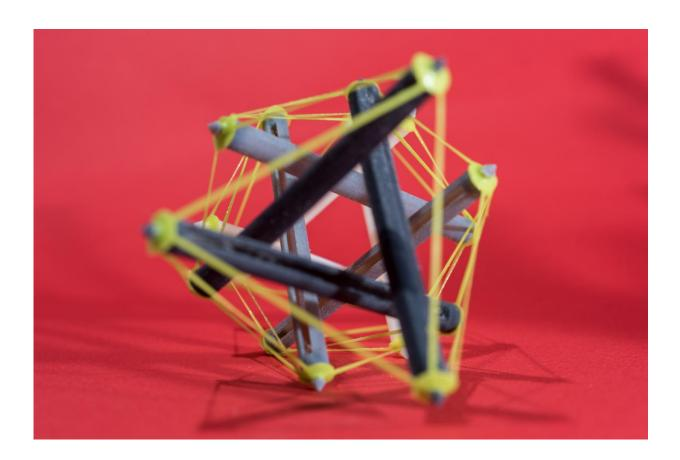
Researchers at Georgia Tech 3-D printed an object made with tensegrity, a structural system of floating rods in compression and cables in continuous tension. Credit: Rob Felt
