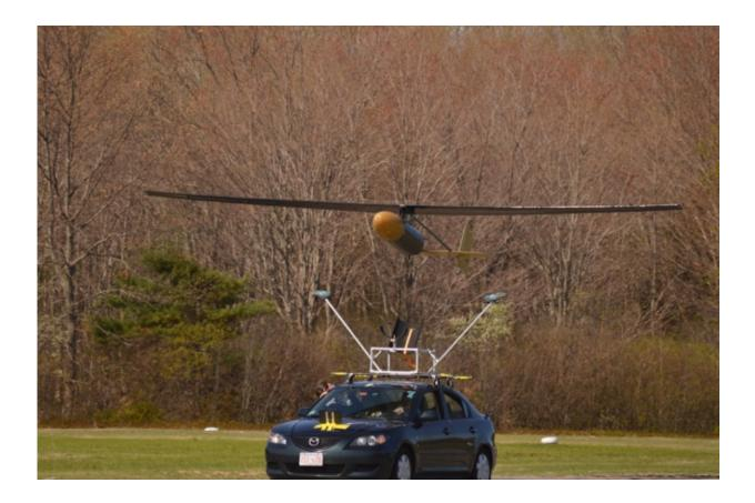
JHO first flight, May 4, 2017 at Plum Island (Mass.) Airport. The aircraft is launched from a moving vehicle. Credit: Veronica Padron/MIT
