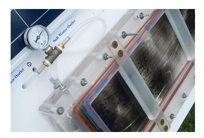
This scaled-up test bed of NEWT's direct solar desalination technology uses carbon black nanoparticles that convert as much as 80 percent of sunlight energy into heat. Results from an earlier prototype showed the technology could produce as much as six liters of freshwater per hour per square meter of solar membrane. Credit: Jeff Fitlow/Rice University
