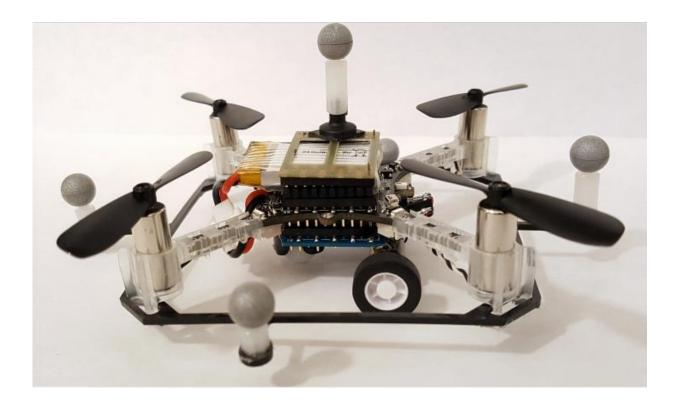
One of the researchers' quadcopter drones with wheels is shown. Credit: Brandon Araki/MIT CSAIL
