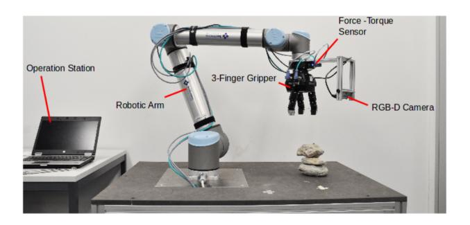
An overview of the used hardware setup: a ROBOTIQ 3-finger gripper, a FT150 force torque sensor, and a Intel RealSense SR300 RGB-D camera are attached to a UR10 arm. Credit: Fadri Furrer
