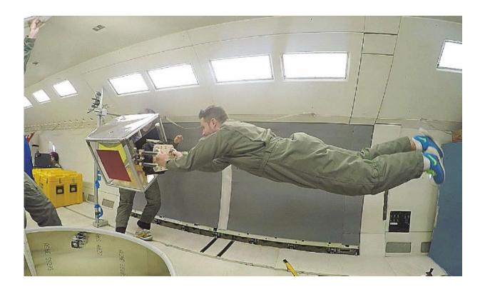
Scientists tested their robotic gripper on NASA's reduced gravity aircraft, the Weightless Wonder. Credit: Jiang et al., *Sci. Robot.* 2, eaan4545 (2017)
