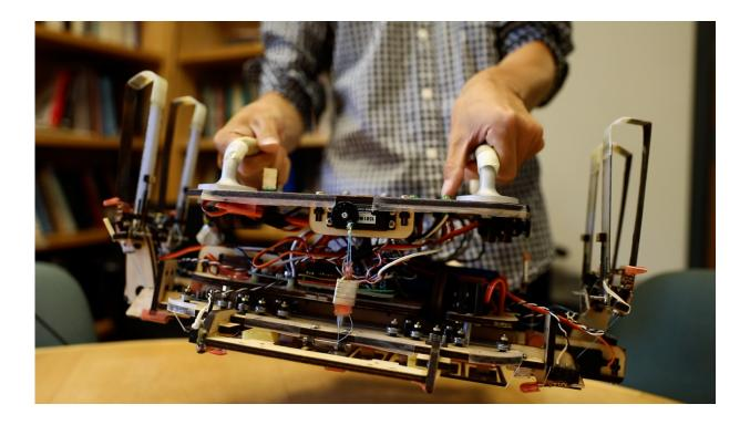
Close up of the robotic gripper made by the Cutkosky lab at Stanford University. The gripper is designed to grab objects in zero gravity using their gecko-inspired adhesive. Credit: Kurt Hickman/Stanford News Service
