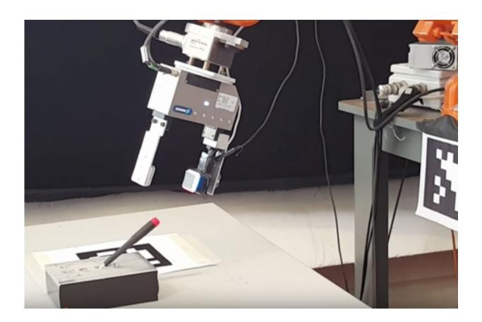
A GelSight sensor attached to a robot's gripper enables the robot to determine precisely where it has grasped a small screwdriver, removing it from and inserting it back into a slot, even when the gripper screens the screwdriver from the robot's camera. Credit: Robot Locomotion Group at MIT
