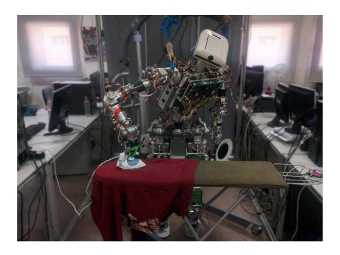
Experimental setup for full-sized humanoid robotic ironing with 3D perception and force/torque feedback. Credit: arXiv:1706.05340 [cs.RO]
