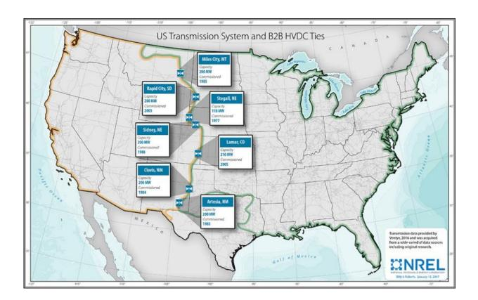
This map shows the country's three primary power grids—the Eastern Interconnection, the Western Interconnection and the Electric Reliability Council of Texas—and the seven small connections between the eastern and western grids. Credit: NREL
