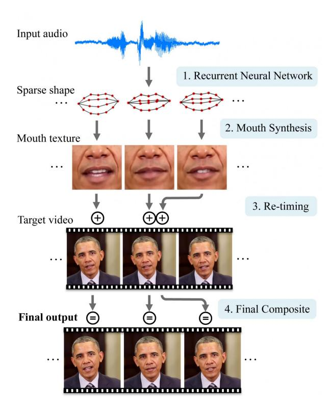
A neural network first converts the sounds from an audio file into basic mouth shapes. Then the system grafts and blends those mouth shapes onto an existing
