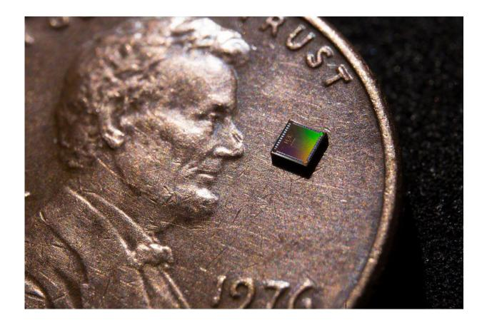
The temperature sensor is integrated into a small chip measuring  $0.15 \times 0.15$  square millimeters in area. Credit: University of California - San Diego
