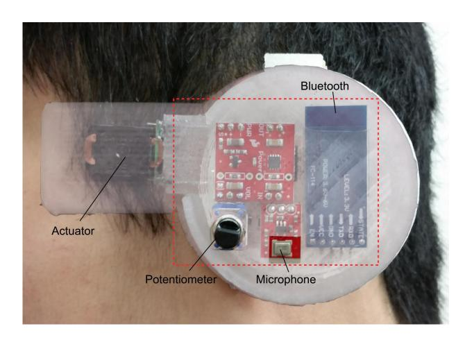
An "earable" sensor can track core body temperature -- a key health indicator -- continuously. Credit: American Chemical Society
