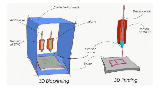
The bioprinting process is performed under sterile conditions and using milder temperatures than are used in 3D plastics printing. Credit: Steffen Harr, Author provided
